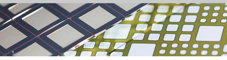
1 Processed SiC wafers featuring JBS-diodes with different device area and current-handling capability
