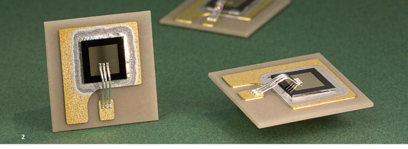
2 High-voltage JBS-diodes soldered and bonded onto ceramic DCBs for high-current applications
