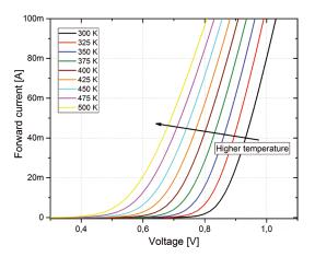
Fig. 3: Temperature-dependence of the conduction mode.
