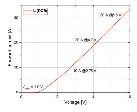
Fig. 1: Forward IV-curve (diode mounted on DCB)
