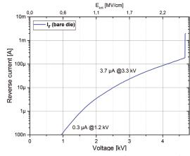
Fig. 2: Reverse IV-curve (3.3 kV diode)
